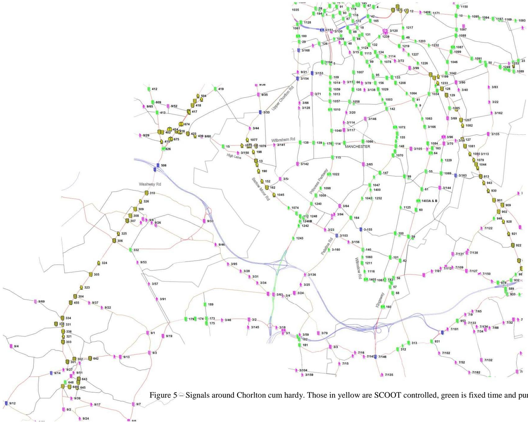
Figure 5 – Signals around Chorlton cum hardy. Those in yellow are SCOOT controlled, green is fixed time and purple VA
