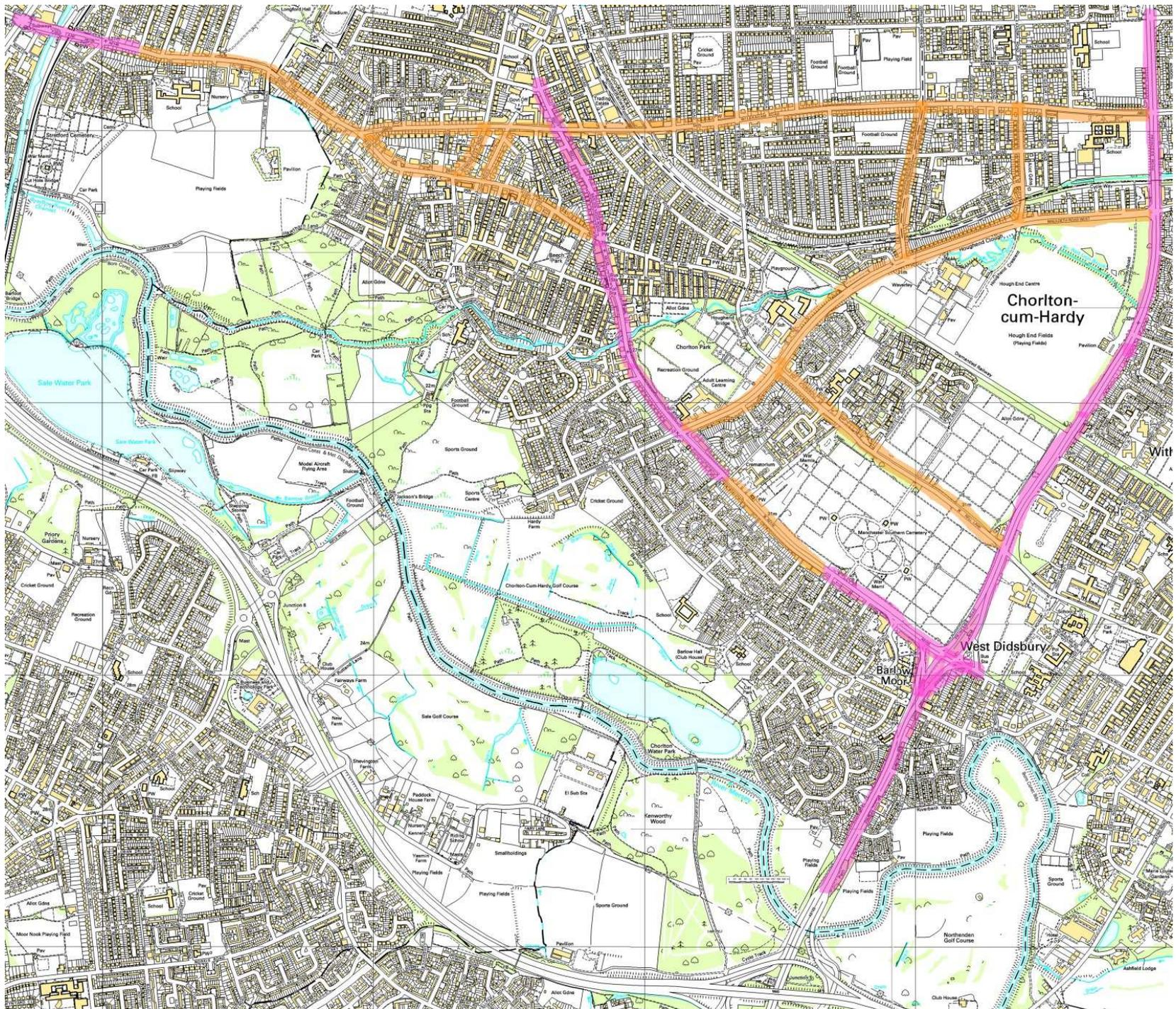
Figure 3 – Road network modelled. Roads operated under SCOOT are marked in purple
